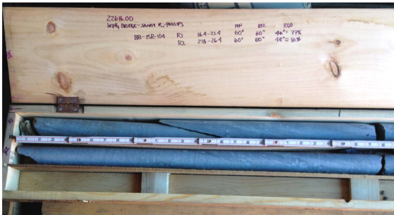
Photo 5: Core box containing rock core from test boring BB-PSR-104 - left side of core box (top portion of cores). From top to bottom 1) BB-PSR-104, R-1; 2) BB-PSR-104, R-2.
