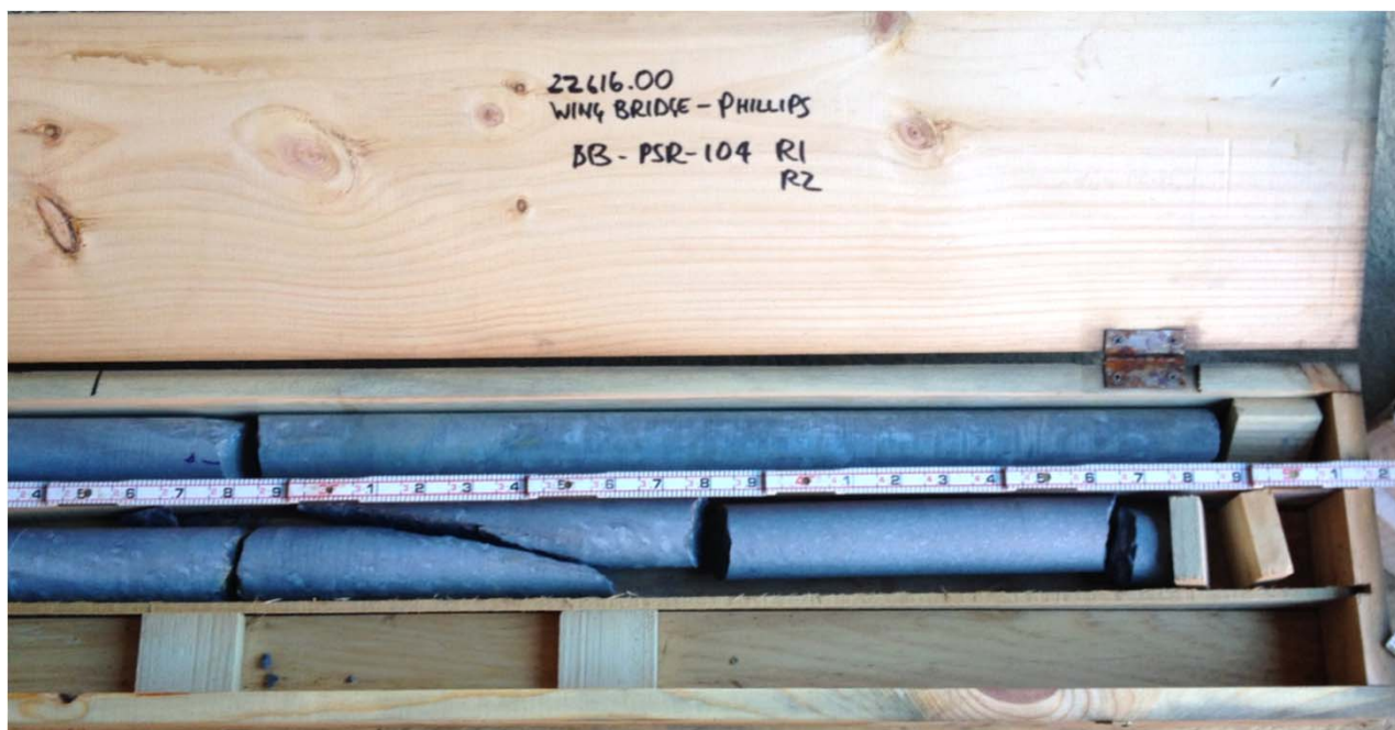
Photo 6: Core box containing rock core from test boring BB-PSR-104 - right side of core box (bottom portion of cores). From top to bottom 1) BB-PSR-104, R-1; 2) BB-PSR-104, R-2.
