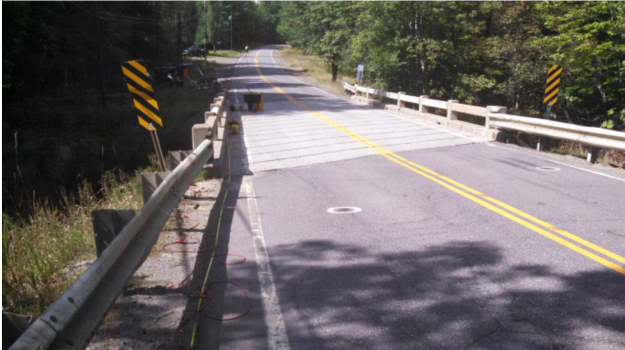
Photograph of Line 1 across the Wing Bridge, looking west. Geophones are planted in the gravel shoulders on either side of the bridge. The seismograph is located in the center of the bridge.
