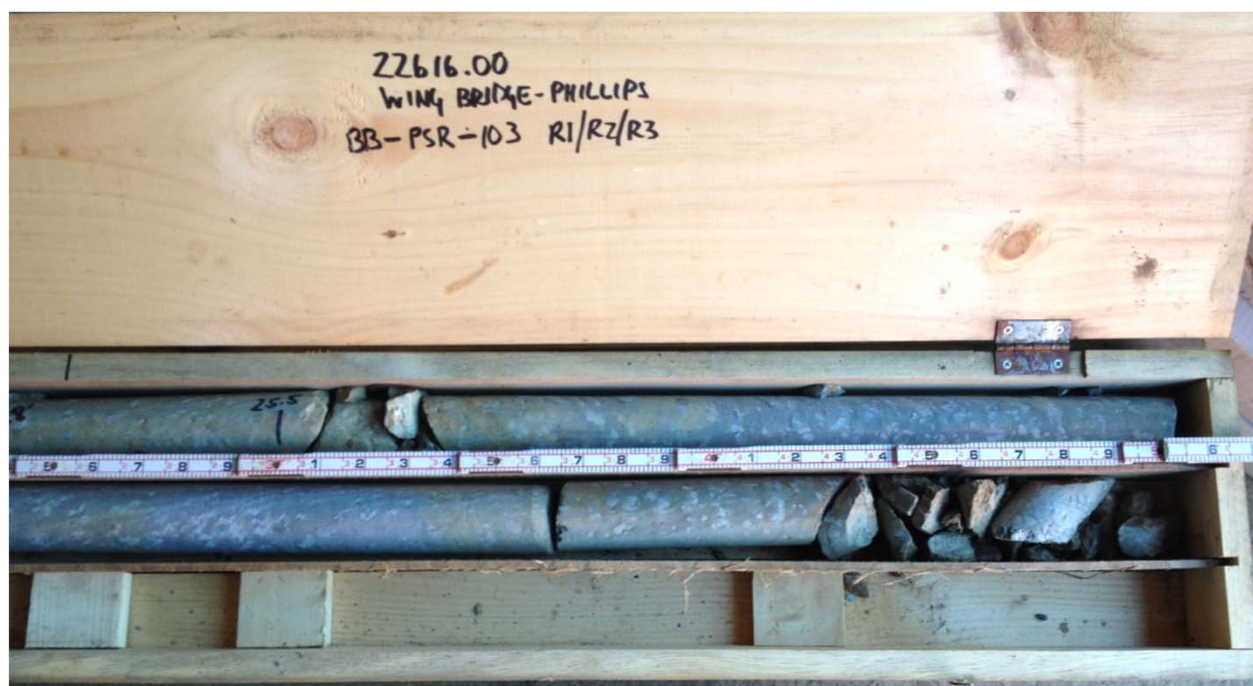
Photo 4: Core box containing rock core from test boring BB-PSR-103 - right side of core box (bottom portion of cores). From top to bottom 1) BB-PSR-103, R-1 and R-2; 2) BB-PSR-103, R-3.
