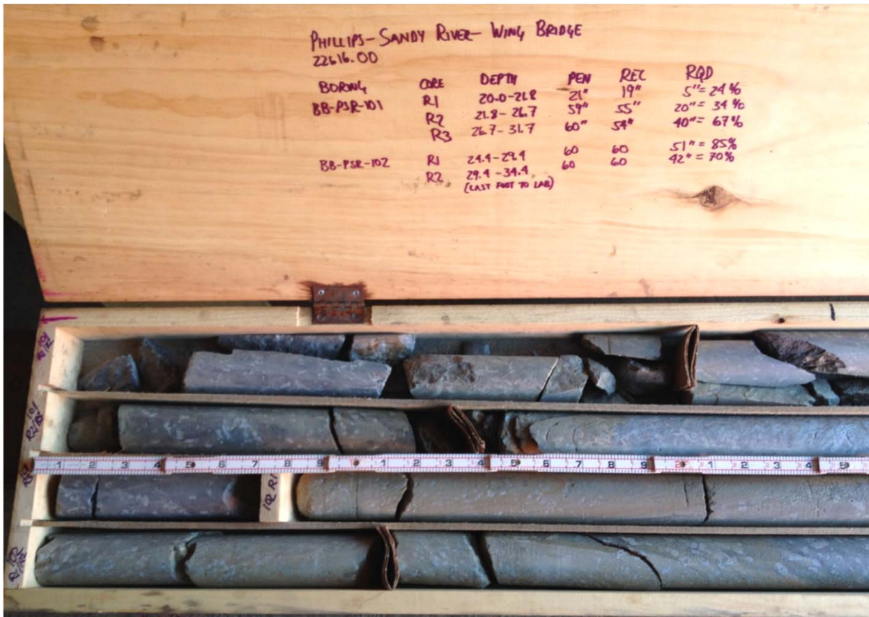
Photo 1: Core box containing rock core from test borings BB-PSR-101 and BB-PSR-102 - left side of core box (top portion of cores). From top to bottom 1) BB-PSR-101, R-1 and R-2; 2) BB-PSR-101, R-3; 3) BB-PSR-102, R-1; 4) BB-PSR-102, R-2.
