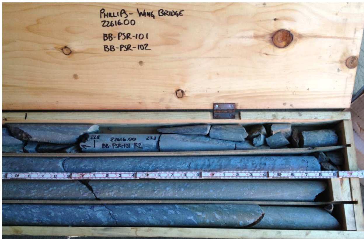
Photo 2: Core box containing rock core from test borings BB-PSR-101 and BB-PSR-102 - right side of core box (bottom portion of cores). From top to bottom 1) BB-PSR-101, R-1 and R-2; 2) BB-PSR-101, R-3; 3) BB-PSR-102, R-1; 4) BB-PSR-102, R-2.
